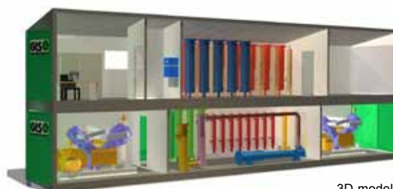
3D-model van GPP26T, 800Nm 3 /hr biogas
